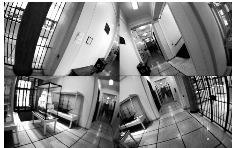
Four Pointgrey Firefly MV Cameras (640x480 8-bit grayscale images) FOV: 360° (h) x 90° (v)
